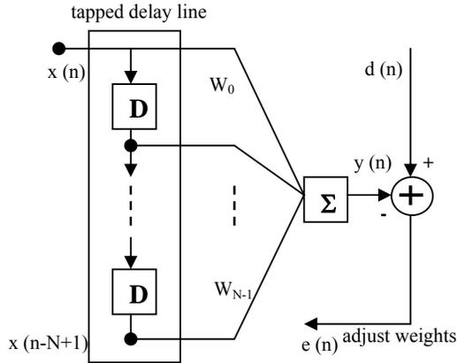
Fig. 4 Adaptive filter block diagram
