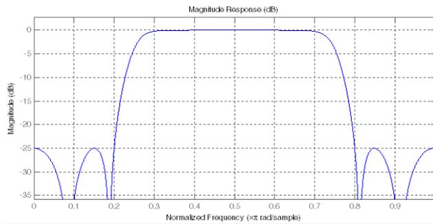
Fig. 6 Filter response curve of frequency versus magnitude (dB)
