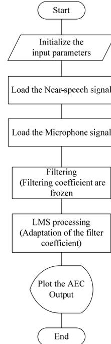
Fig. 5 Flowchart of the AEC system
